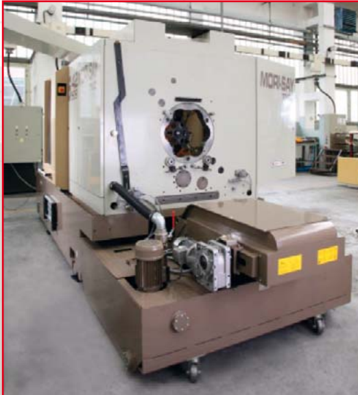
Mobile sedimentation tank inserted into the machine base - traditional solution by the TAJMAC-ZPS
